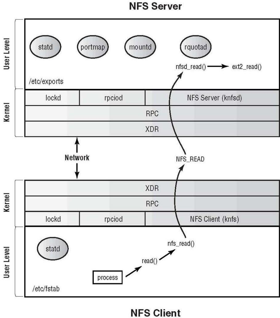
**Figure 1.1: The components of an NFS system [F0101.eps]**
