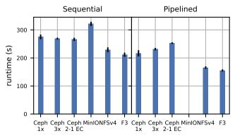
*Figure 9: Runtime of Cutadapt + Trimmomatic pipeline. F3 was layered on top of an unreplicated CephFS volume.*
