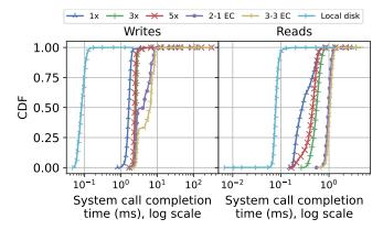
Figure 4: CDFs of read and write system call latencies, for different storage configurations. We used log scale for the x-axis because the system calls exhibited long tails at higher replication degrees.
