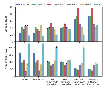
Figure 6: Mean latencies and bandwidths of Ceph, NFS, MinIO, and F3. "Ceph  $1 \times$ " and "Ceph  $3 \times$ " are configured with  $1 \times$  and  $3 \times$  replication, respectively. "Ceph 2-1 EC" uses erasure coding (data split into two data chunks and one coding chunk). F3 was layered on top of an unreplicated CephFS volume.
