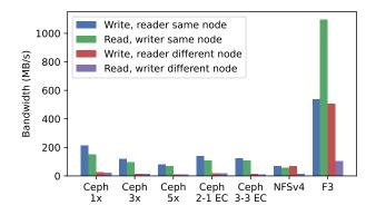
Figure 7: Comparison of read-while-write performance, when readers and writers are on the same or different nodes. For CephFS, having the reader and writer on different nodes significantly degrades both read and write performance. MinIO is absent from this experiment due to its inability to read and write data concurrently. F3 was layered on top of an unreplicated CephFS volume.
