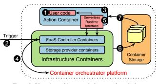
Figure 1: Blueprint architecture of edge serverless platform
