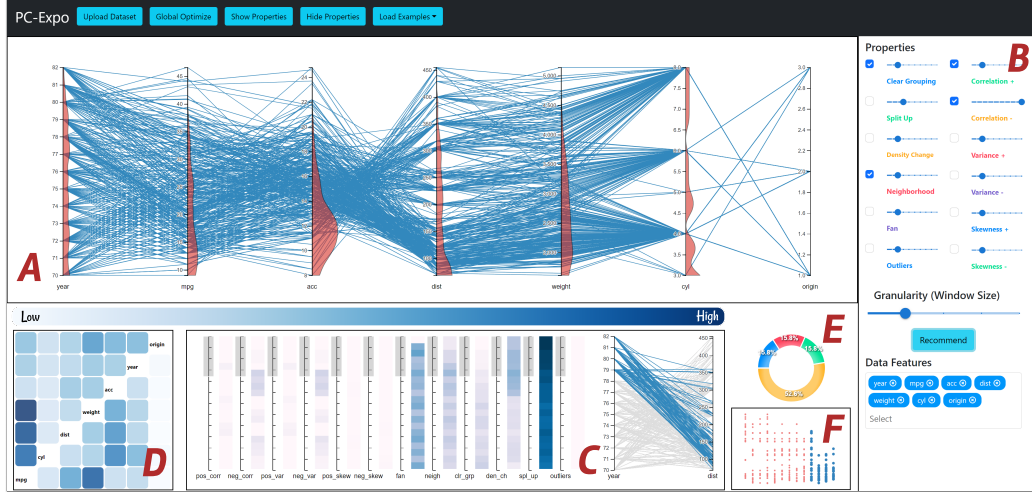
Figure 6.2: PC-Expo is a real-time all-in-one Parallel Coordinate Plot (PCP) axes reordering framework. PC-Expo detects local properties in high-dimensional data that can be used to reorder the PCP axes automatically or with human-in-the-loop (HIL) interactions A. We have implemented detectors for the 12 most common data properties used to reorder PCPs, shown on the properties panel B. Users can create their own optimization scheme using a weighted sum of these properties, by selecting respective properties and weights from (B), summarized as a donut chart E for automated axes reordering. PC-Expo also supports HIL axes reordering via a heatmap and local views D, C, and F. D summarizes the weighted sum of user-selected properties detected locally for each axis pair. C shows where these visualization properties were detected for a particular axis pair, with a linked scatterplot F for visualizing the 2D data points. Users can manually reorder the axes using these local views by clicking on D sequentially. The granularity slider in B lets users control the size of local regions used to detect the properties. Area charts next to PCP axes in A show the local regions where the properties selected on (B) are detected on the axis.
