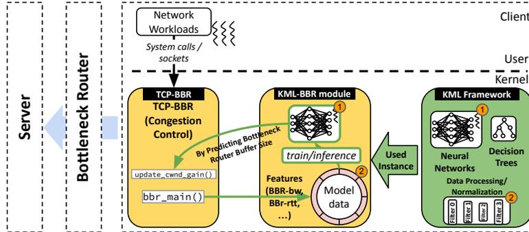
Figure 6.2: KML BBR Architecture
