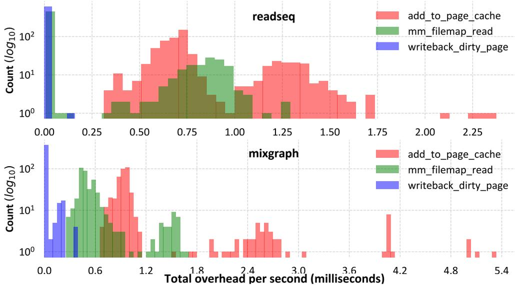
Figure 5.7: Distribution of total data collection overhead (milliseconds) in every second when `readseq` and `mixgraph` workloads are running.
