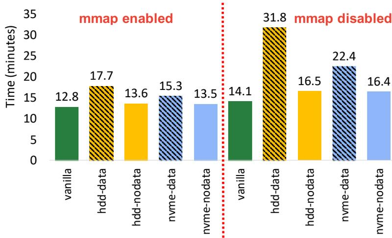
Figure 4.6: Results of HDD vs. NVMe devices used to record traces, along three dimensions: (i) capturing traces on HDD vs. NVMe (yellow vs. blue bars); (ii) capturing with data buffers vs. only system-call metadata (hatched pattern vs. clear); and (iii) capturing LevelDB using `mmap` vs. `read/write` (separated by vertical dotted line).
