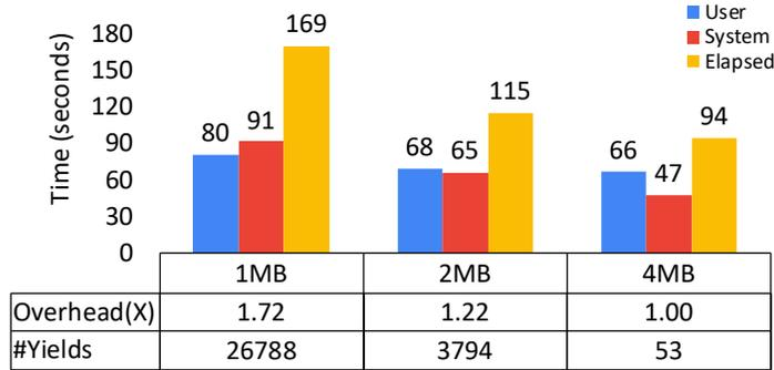
Figure 4.5: RA-LTTng blocking-mode overheads for tracing LevelDB `db_bench` with its default database configuration. We used 3 different RA-LTTng sub-buffer sizes (4MB, 2MB, and 1MB); we show user, system, and elapsed times for each experiment. The table below also shows the elapsed time overheads relative to the 4MB baseline and the number of yield calls executed.
