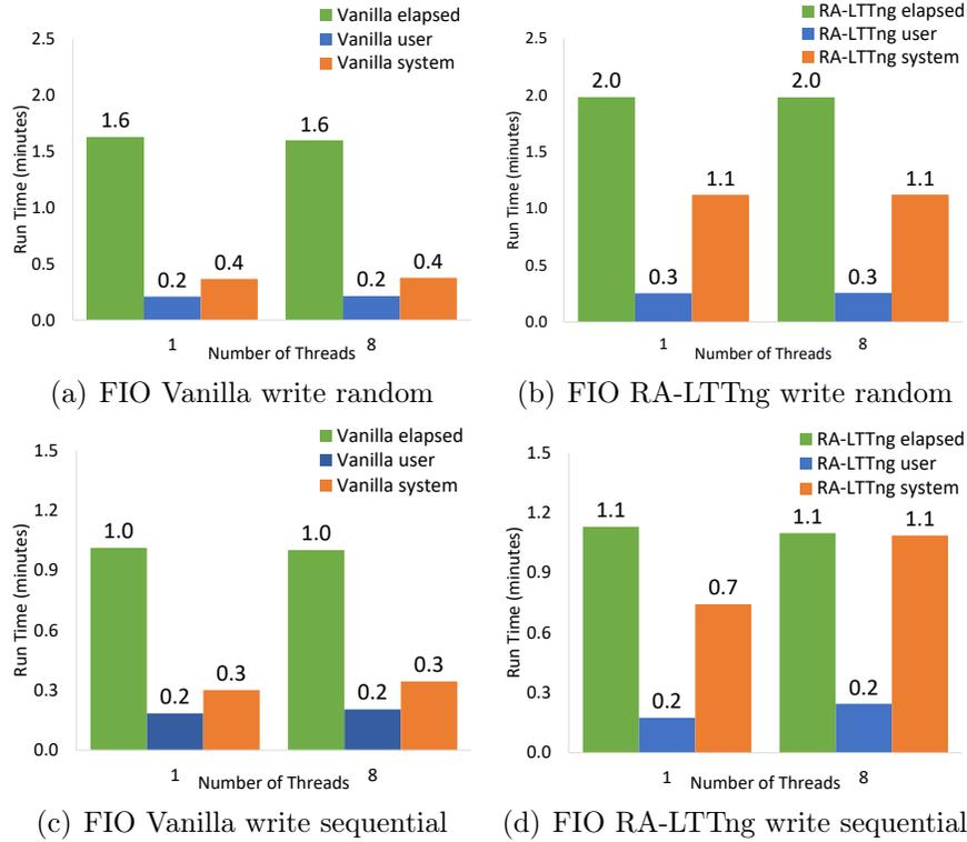
Figure 4.3: FIO random and sequential write times in minutes (elapsed, user, and system). Vanilla denotes FIO without tracing; RA-LTTng denotes FIO with full tracing enabled. Note that the Y-axis scales differ between the random and sequential pairs of figures.
