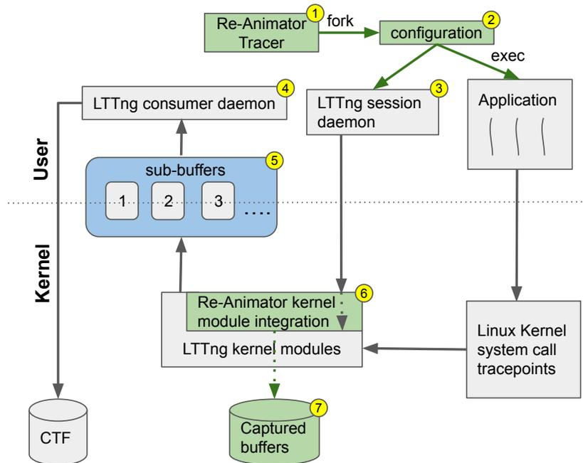
Figure 4.1: LTTng architecture using Linux kernel tracepoints. Green boxes denote our additions or changes. Our wrapper (1) launches the LTTng configurator (2), which invokes an LTTng session daemon (3) to control the operation and the consumer daemon (4) to collect events. LTTng tracepoints place events into sub-buffers (5) and invoke Re-Animator, which collects data buffers and writes them to a separate disk file (7).
