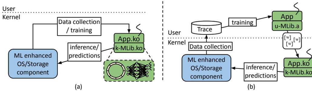
Figure 5.1: Two different operational modes that we built to achieve a high efficiency ML framework for tuning OS-level storage systems: (a) kernel space training and inference and (b) offline user space training and kernel space inference.
