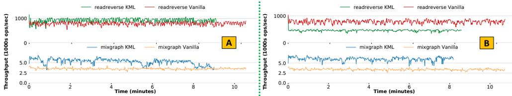
Figure 5.10: Mixed workloads results on a timeline, comparing the readahead neural network model running on per-file basis ('A', left) vs. per-disk basis ('B', right).
