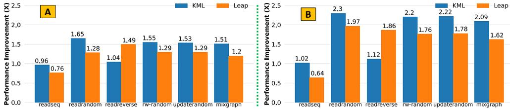
Figure 5.15: Performance improvement comparisons between LEAP [10] and KML for RocksDB benchmarks on NVMe-SSD ('A', left) and SATA-SSD ('B', right).
