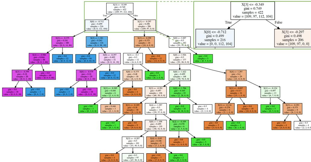
Figure 5.5: A readahead decision tree is built to classify RocksDB workloads running on a NVMe-SSD backed device. Colors denote workload classes: orange for readrandom workload, green for rw-random, blue for readseq, and purple for readreverse.
