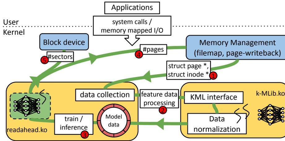
Figure 5.2: KML kernel space training and inferencing architecture.
