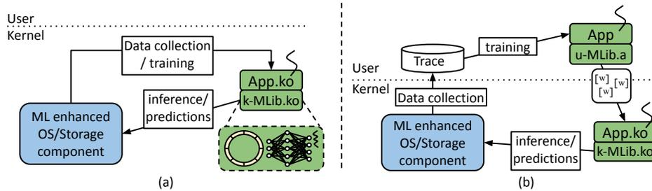
Figure 5.1: Two different operational modes that we built to achieve a high efficiency ML framework for tuning OS-level storage systems: (a) kernel space training and inference and (b) offline user space training and kernel space inference.
