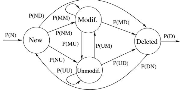
Figure 4: Markov model for handling file states. State transitions are denoted by the first letters of the source and destination states. For example, NM denotes a New $\rightarrow$ Modified transition and  $P(NM)$  is the transition's probability.
