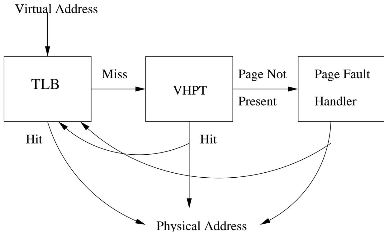
Figure 8: Virtual to Physical address conversion using TLB and VHPT
