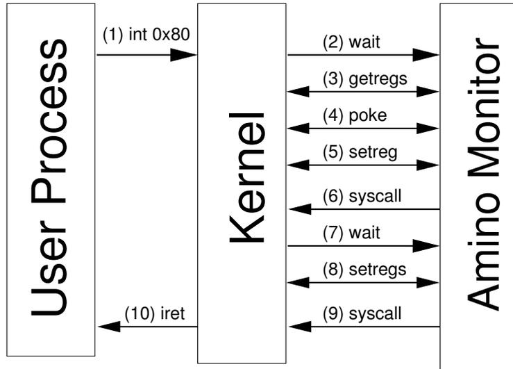
Figure 3.2: *ptrace* primitives used to handle a `read` system call. Arrows indicate control transfer. Double arrows indicate that the function was called and returned immediately.
