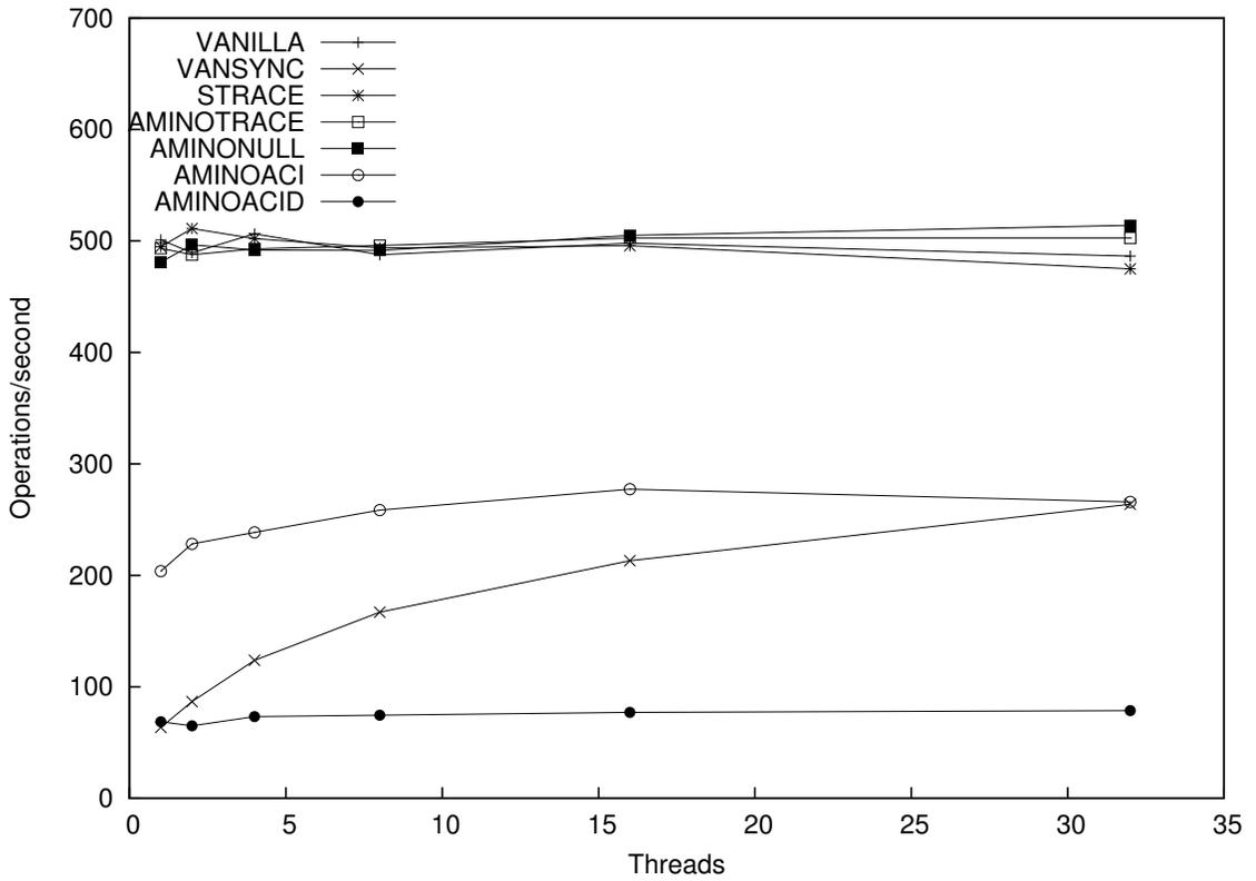
Figure 5.15: Data micro-benchmark results: Multi-threaded random write.
