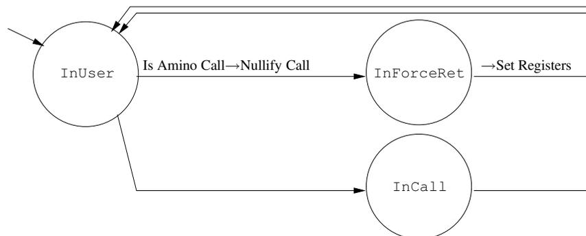
Figure 3.3: *The monitor has 17 states that determine its actions after `wait` returns. This diagram shows three of those states: `INUSER`, `INCALL`, and `INFORCERET`. The edges are labeled with implications. If the antecedent is true, then the edge is followed after the actions in the consequent are performed. Unlabeled edges are followed unconditionally.*
