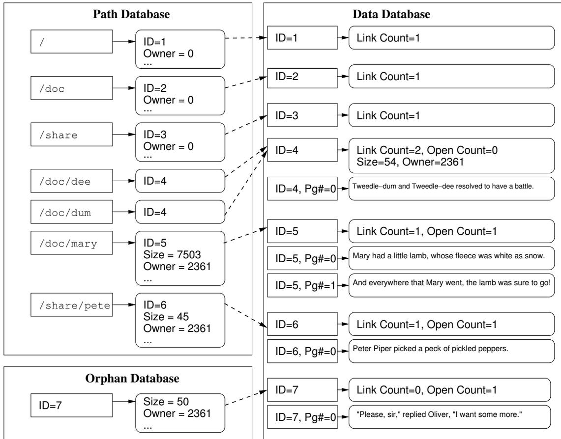
Figure 2.1: A sample Amino file system. Within a database, keys (rectangles) and data (rounded rectangles) are connected by solid arrows. Logical relationships between databases are denoted by dashed arrows.
