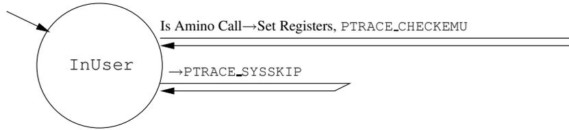
Figure 3.8: *Figure 3.3 assumes the standard `ptrace` interfaces. Our new primitives reduce the number of states and transitions needed for many calls. `PTRACE_CHECKEMU` removes the need for the `INFORCERET` state and `PTRACE_SYSSKIP` removes the need for the `INCALL` state.*
