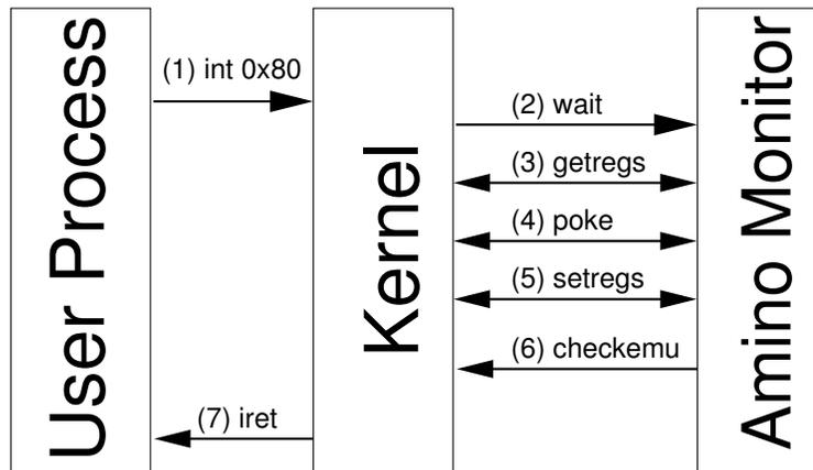
Figure 3.7: *The `PTRACE_CHECKEMU` call reduces the number of `ptrace` primitives required for servicing a system call compared to the standard `ptrace` primitives shown in Figure 3.2.*
