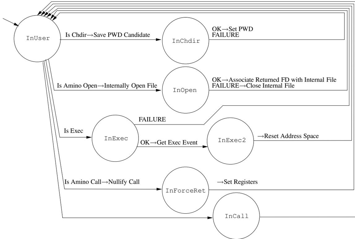
Figure 3.4: Most of the 17 monitor states are for specific calls. Using the same notation as Figure 3.3, this state diagram shows the transitions for `open`, `chdir`, and `exec`.
