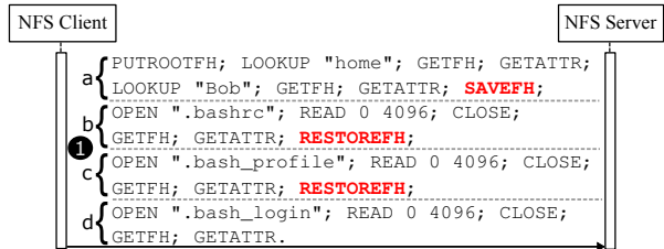
Figure 3: One NFS compound that reads three files. The operations can be divided into four groups: (a) sets the current and saved filehandle to /home/Bob ; (b), (c), and (d) read the files .bashrc , .bash_profile , and .bash_login , respectively. SAVEFH and RESTOREFH (in red) ensure that the CFH is /home/Bob when opening files. The reply is omitted.
