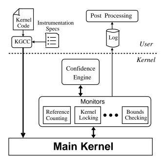
Figure 6.1: Architectural overview of the Aristotle system. KGCC instruments kernel code with monitoring calls. During the execution of the instrumented kernel, the monitoring calls invoke individual monitors to dynamically verify system properties.
