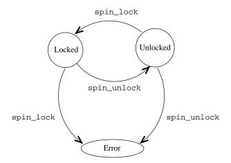
Figure 2.1: Example of an Application Level Protocol that should be satisfied in program code. During normal operation, the system can be in one of two states: Locked or Unlocked . Calls to spin \_lock and spin \_unlock cause transitions between these states. Any other transition results in an error.
