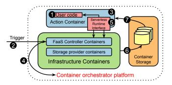
Figure 1: Blueprint architecture of edge serverless platform
