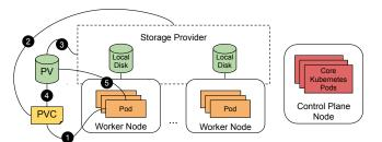
Figure 1: Basic topology of a Kubernetes cluster, with a single control plane node, multiple worker nodes, and a storage provider which aggregates local storage attached to each worker node. Also shows the operations and resources involved in providing a Pod with storage.
