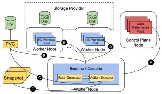
Figure 2: CNSBench overview with its components in blue
