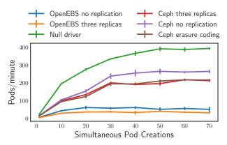
Figure 5: Volume creations and attachments per minute, for different numbers of simultaneous operations. The vertical lines at each point shows the standard deviation for volume creation and attachment rate at that point.
