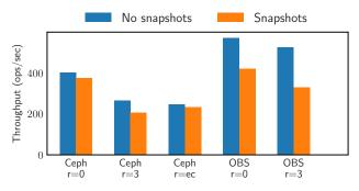
Figure 6: Effect of snapshotting on I/O workload. r=0 indicates zero volume replicas, r=3 indicates three volume replicas, and r=ec indicates erasure coding.
