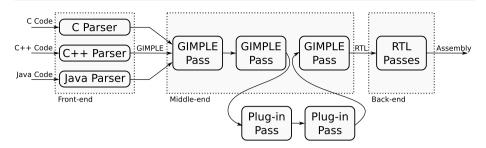
Fig. 1 A simplified view of the GCC compilation process
