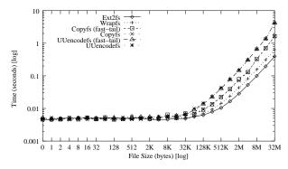
Figure 7: Copying files into a tested file system. As expected, uuencodefs is costlier that copyfs, wrapfs, and ext2fs. Fast-tails do not make a difference in this test, since we are not appending multiple times.
