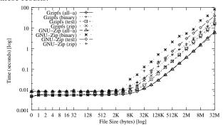
Figure 8: Comparing file copying into gzipfs (kernel) and using GNU zip (user-level) for various file types and sizes.
