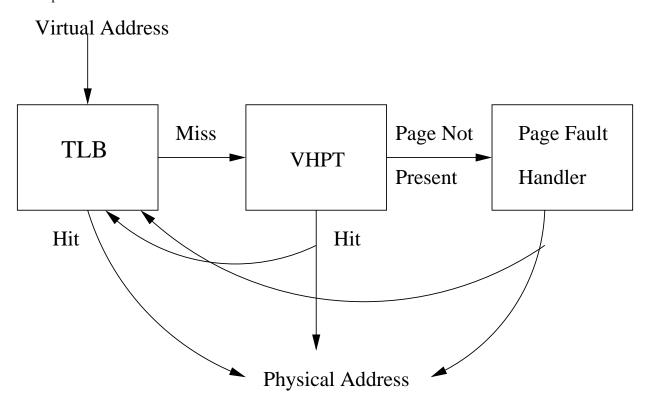
Figure 8: Virtual to Physical address conversion using TLB and VHPT
