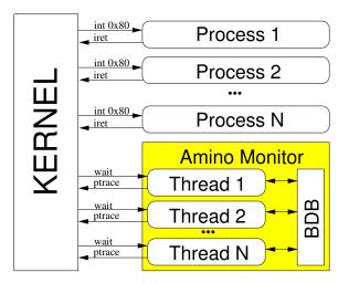
Figure 3.1: The Amino monitor can trace an arbitrary number of processes. Each application process is traced by a separate thread within the monitor. At system call entry, the kernel signals the monitor via the wait system call. Amino manipulates the monitored processes' state with ptrace primitives. BDB executes within the monitor's address space and uses standard system calls.
