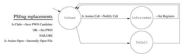
Figure 3.3: The monitor has 17 states that determine its actions after wait returns. This diagram shows three of those states: INUSER, INCALL, and INFORCERET. The edges are labeled with implications. If the antecedent is true, then the edge is followed after the actions in the consequent are performed. Unlabeled edges are followed unconditionally.
