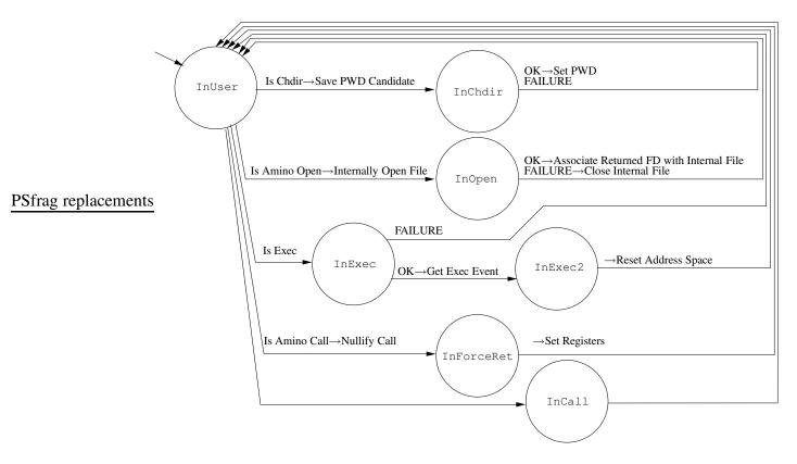
Figure 3.4: Most of the 17 monitor states are for specific calls. Using the same notation as Figure 3.3, this state diagram shows the transitions for open, chdir, and exec.
