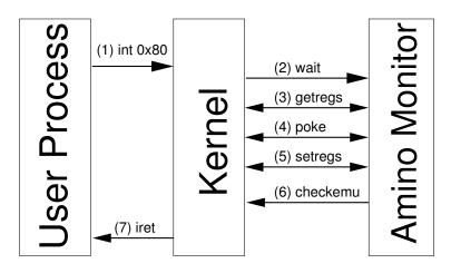
Figure 3.7: The PTRACE\_CHECKEMU call reduces the number of ptrace primitives required for servicing a system call compared to the standard ptrace primitives shown in Figure 3.2.
