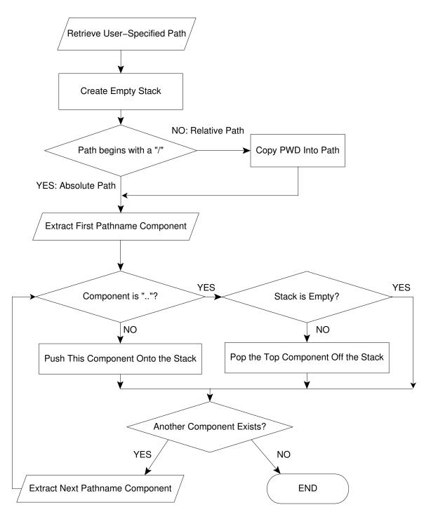
Figure 3.5: The monitor uses stacks to represent path name components. When a new component is encountered, it is pushed onto the stack. When a "..." is encountered a component is popped off the stack.
